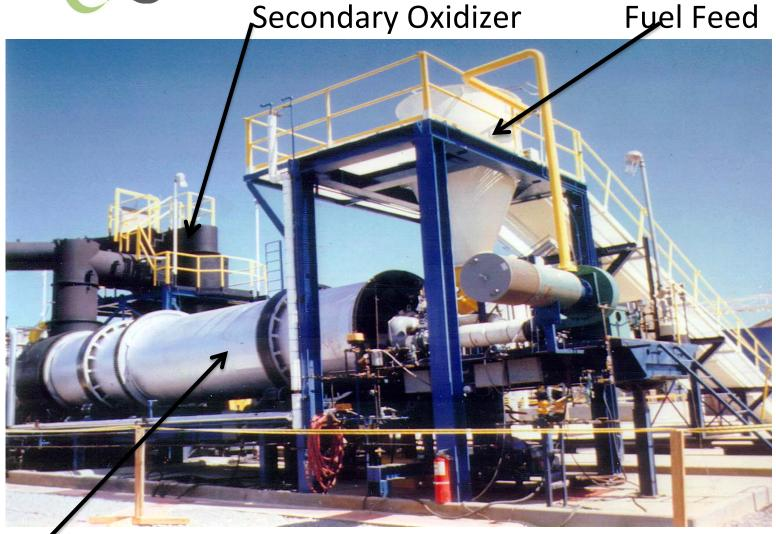
Rotary Kiln (Primary Oxidizer)
